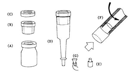
Technique: Amidites were prepared in sealed bottles (A) and injected to the column containing support through "press-in" teflon cap (B) equipped with pressed-on membrane coated aluminium seal (C). Bottom of the column (D) was closed with rubber sleeve stoper (E). During coupling the column was rotated (F) (inlet of rotary evaporator could be used). Other reagents were delivered in flow-stop flow mode to the open column with outlet made from silicon rubber tube (G). Device allow easy scale-up.
